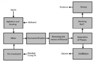
Fig. 2. Process of Transesterification
