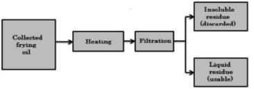
Fig.1. Pre-treatment process of cooking oil
